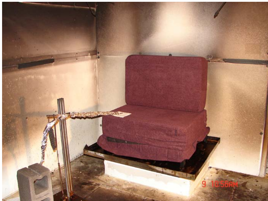
Photo 2. Smoldering ignition of a chair mock-up. The heat source was removed after smoldering initiation (about 6 min).
