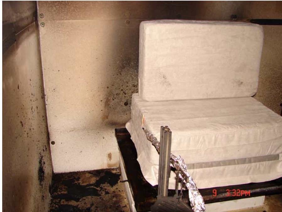
Photo 1. Flaming ignition of a chair mockup. The ignitor was removed after 40 s.
