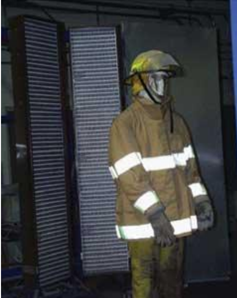
(3) An instrumented mannequin in front of electric radiant panels.
