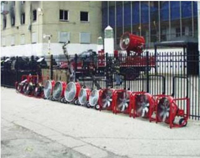
(5) A wide variety of portable fans were used during the Toledo and Chicago high-rise experiments.
