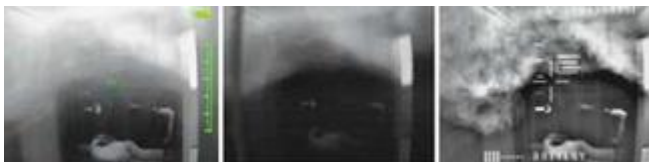
(1) Comparison of three thermal imaging camera detector technologies of the same fire environment at the same time: (left to right) vanadium oxide (VOx), amorphous silicon (ASi), and barium strontium titanate (BST). (Photos courtesy of NIST.)
