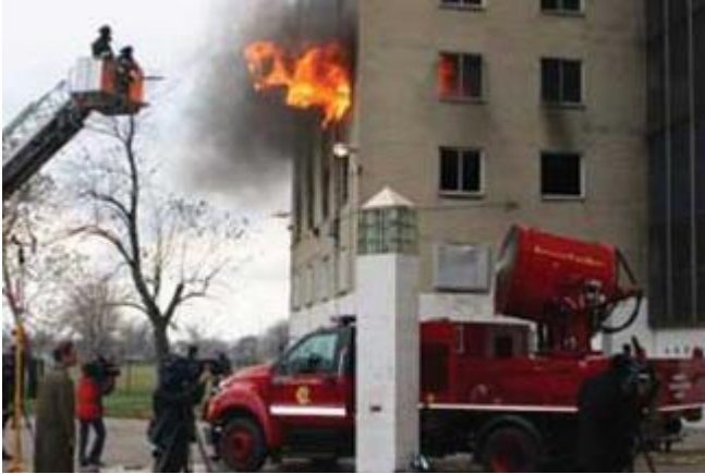
(4) The Chicago Fire Department's truck-mounted fan pressurizes the first floor and the stairwell and forces the fire back through the fire apartment and out the window.
