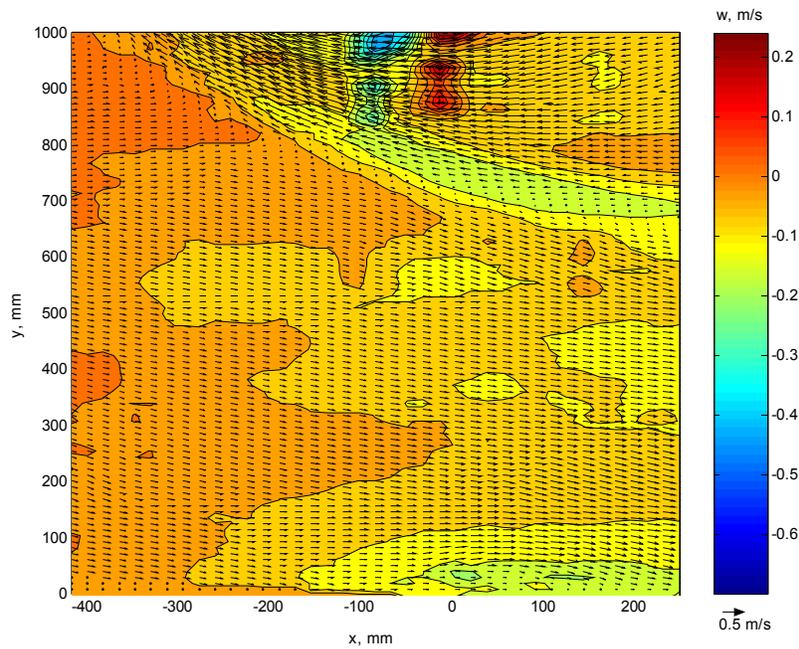
**Figure 2 Mean velocity field through doorway centerline,  $z = 0$  mm. Color map represents  $w$  velocity component, vectors represent  $u$  and  $v$  velocity components.**
