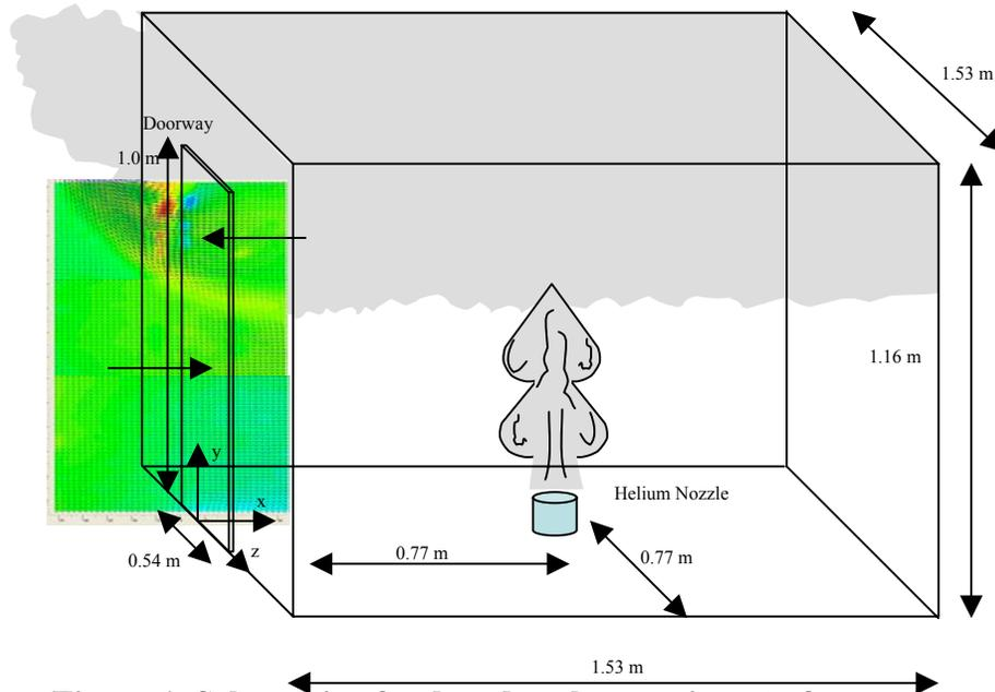
**Figure 1 Schematic of reduced-scale experiment of an enclosure fire analogue**
