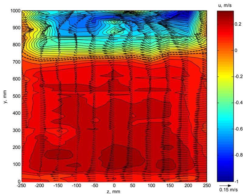
**Figure 3 Mean velocity field across doorway plane,  $x = -14$  mm. Color map represents  $u$  velocity component, vectors represent  $v$  and  $w$  velocity components. The color map is interpolated between vertical slices. Neutral plane is indicated by heavy dashed lines outlining adjacent contours where flow changes direction.**
