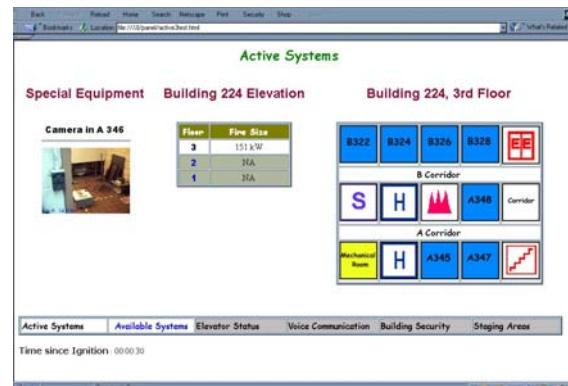
**Figure 3 - NIST prototype fire service interface**
