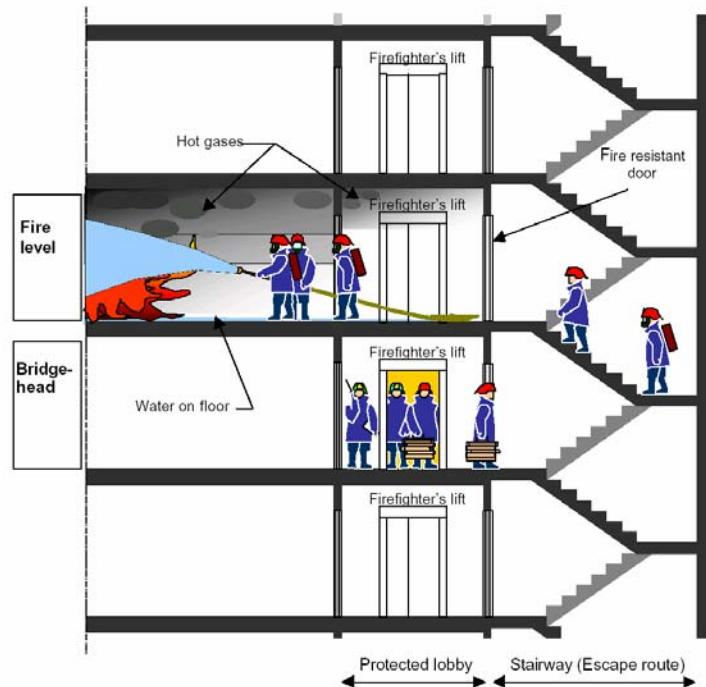
**Figure 4 - firefighter lifts carry people and equipment to the floor below the fire with attack staged from the stairs<sup>9</sup>**
