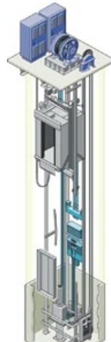
**Figure 1 - Typical electric elevator**
