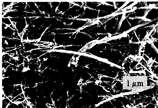
Figure 1. SEM photomicrograph of MWNT dispersion in the poly(propylene) composite after solvent removal.
